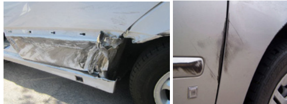
Figure 5: Examples of rubber transfer evidence.
