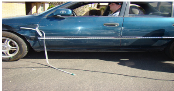
Figure 1: Typical sideswipe damage with side view mirror rotated rearward (overtaking vehicle).
