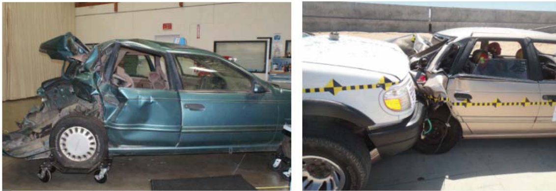
Figure 2: Comparison of Accident Vehicle Right Side Damage (Blue Vehicle) with Confirmation Test Vehicle.
