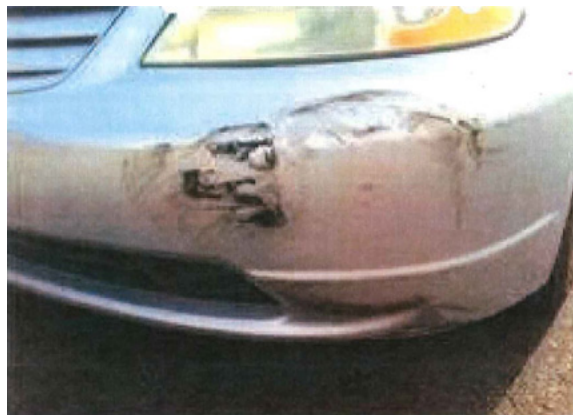
Figure 2: Material flow from vehicle passing from passenger's to driver's side.
