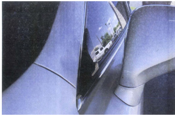
Figure 4: Mirror strike from forward rotating mirror housing.
