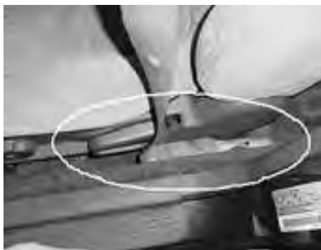
Figure 2, Belt Fuse Caught Beneath Seat
