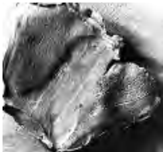
Class characteristic rifling marks/fingerprint of the barrel marks on the inside of the lead core.
