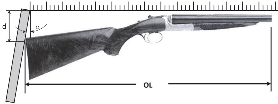
Figure A.1—Misalignment or Squareness Error Between the Measurement Datum and Scale (adapted from [17])
